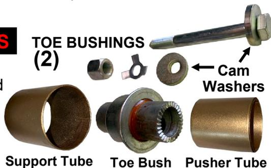
**C** Reconnect Toe arms using the new KMAC D shape bolts and cam washers supplied with the 'tab' lock washers under each nut
